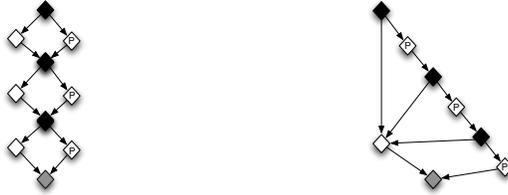
(a) TACO's loop unroll encoding (b) New encoding of loop unrollings
