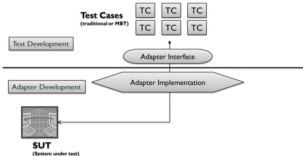
Figure 5 depicts the role of test adapters in the process. Test adapter interfaces are developed and used independently of their implementation. At deployment time, test adapter implementations are associated with adapter interfaces, supporting different implementations with the same logical functionality for different protocol transports and/or operating systems.
