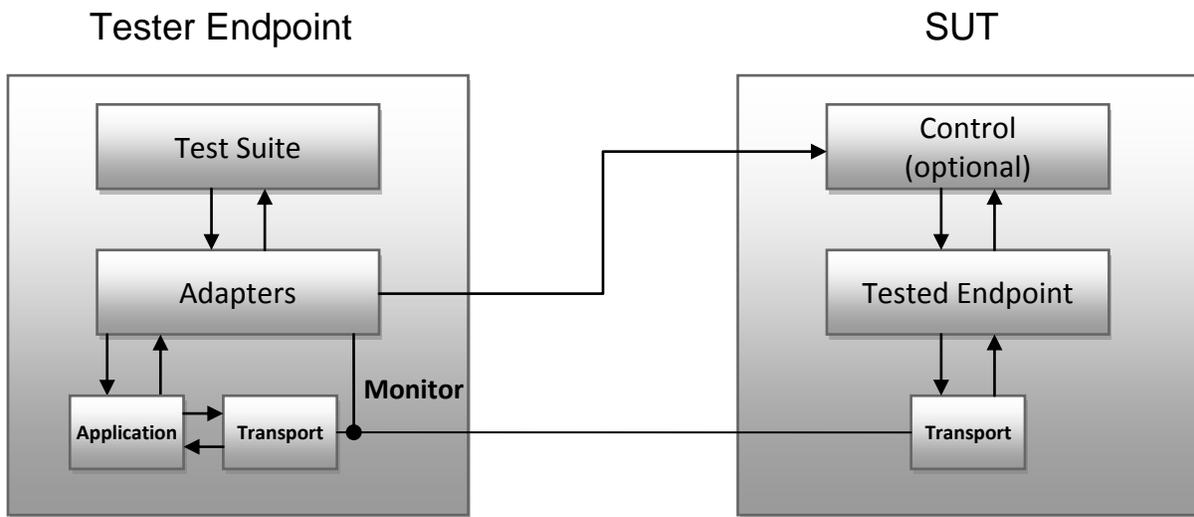
Both approaches use test adapters (described in Section 3) to abstract the access to the SUT and harness for the actual test cases. Both approaches may require, in addition to the operations provided by the tested protocol, some additional control of the tested endpoint, shown in both figures as “Control”.
